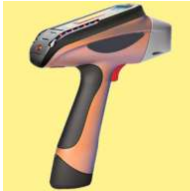
Fig. 2.1.2: Handheld X-ray fluorescence Spectrometer
