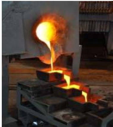
Fig. 1.4.5: Molten gold being poured from a crucible into an ingot mold
