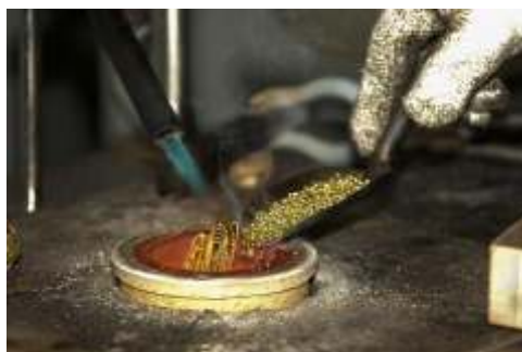
Fig. 1.4.4: gold melting process
