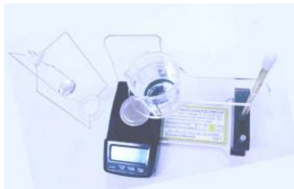
Fig. 2.1.1: Gold testing using specific gravity
