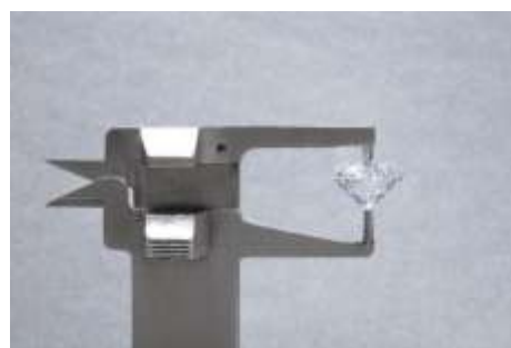
Fig. 1.3.6: Loose big brilliant round diamond is being measure by mm gauge and weight estimator for size
